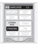
*With multichannel sources* (such as DVDs and digital satellite broadcasts), the **DI DIGITAL** or **DTS** indicator on the front panel lights depending on the source format. Any active Advanced surround or Home THX mode is canceled.
